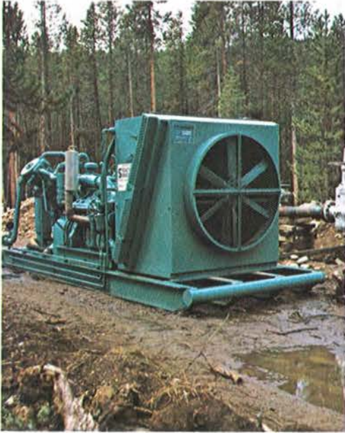
This skid-mounted gas compressor will be installed on a concrete pad to provide pressure for a small gasline.
